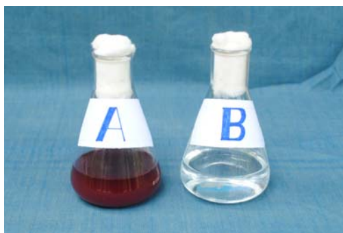
Figure 1: Aqueous silver ions were reduced to silver nanoparticles when added to the biomass of Micrococcus luteus . This was indicated by the change in colour from whitish yellow to brown
