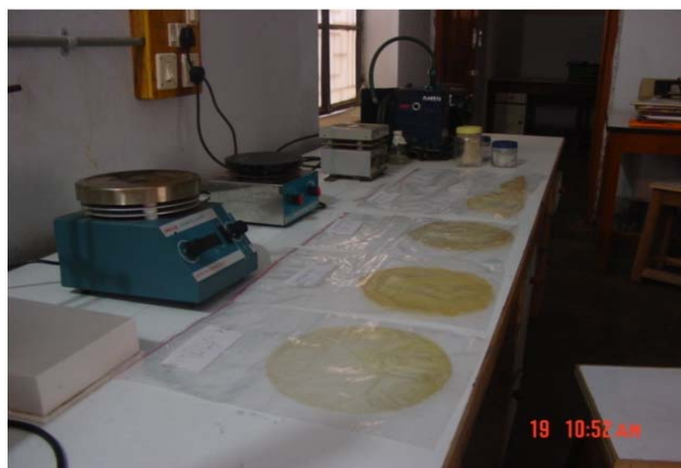
Figure 3. Chitosan films prepared by different casting solvent
