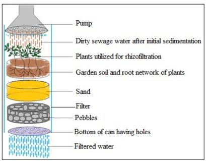
Figure 1: Rhizofiltration apparatus used for water treatment
