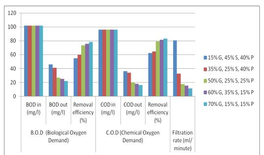
Figure 4: Biological oxygen demand (BOD) and Chemical Oxygen demand (COD) before and after filtration of the effluent. (G= Garden Soil S= Sand P =Pebbles)
