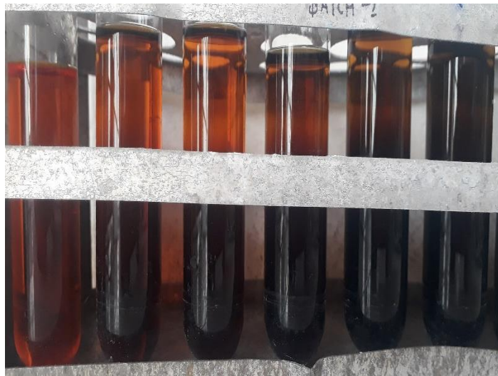
Figure 7: Ethanol estimation using potassium dichromate method
