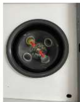
Second spin 3500 RPM for 7 minutes.
