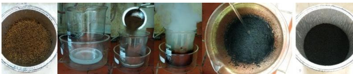
Figure 1: From left-to-right: waste tea carbonization in piranha solution, followed by washing and drying of the product, resulted in a fine carbon powder (namely WTPS) at 32 % yield.
