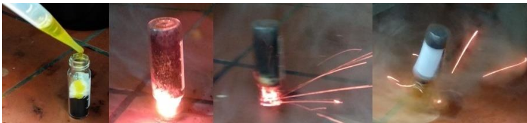
Figure 11: A mini rocket was made of a small glass vial, the aniline-intercalated WTPS and fuming nitric acid \text{HNO}_3 . The glass vial was partly packed with the solid fuel and a small piece of cotton was placed on top of the black powder. Following, fuming nitric acid \text{HNO}_3 was added dropwise until it was fully absorbed by the small piece of cotton. The vial was then flipped upside down to initiate ignition and lift-off the mini rocket within a veil of smoke and sparks.
