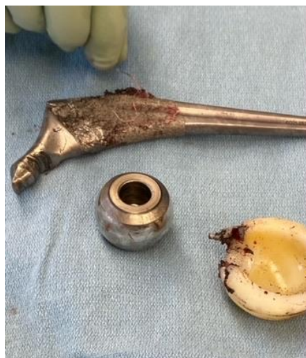
Figure 5: All the components are extracted and demonstrates the “bird beak” appearance of the trunnion as well as the worn polyethylene liner and black discoloration of the femoral head.
