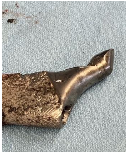
Figure 6: A close view of the “bird beak” appearance of the femoral trunnion.
