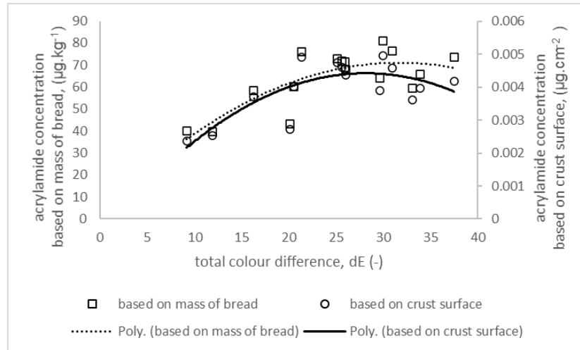
Figure 9: Total colour difference dE vs. acrylamide concentration Ac based on mass of bread and on crust surface area.
